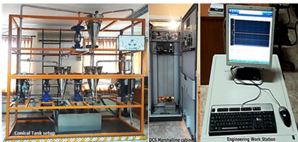
Fig. 7. Proposed pilot plant DCS interfaced two-tank conical system
